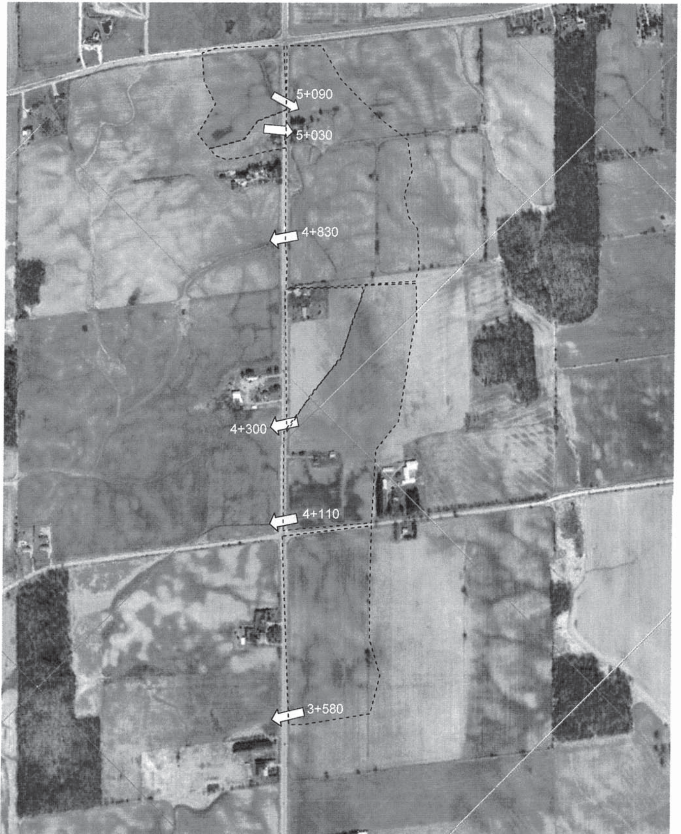
Figure 3. Catchment Areas of Existing Culverts Crossing Mississauga Road (North Half of Study Area)
